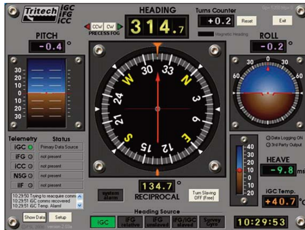
Custom iVP (Intelligent Valve Pack) display, showing iGC heading, pitch and roll.
