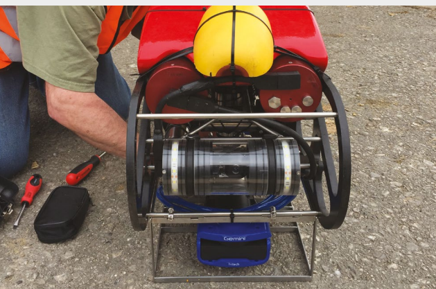
The ROV fitted with the sonar ready for deployment
