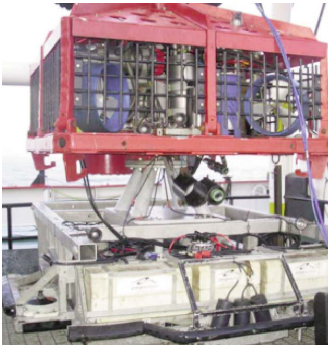
Image of the Atlantic Maritime ROGE-ROV* with the PanGeo Sub-Bottom Imager (SBI) module (as visible) where the Gemini 620pd was mounted along with a PHINS** positioning system.
