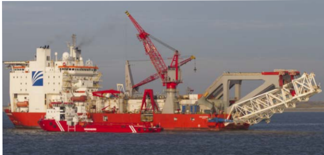
Pipelay vessel with stinger at the rear.
