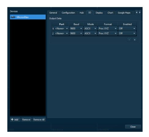
The *IO* tab (shown above) contains the setup options for Remote Communications. This allows the outputting of sensor data to a survey computer.
