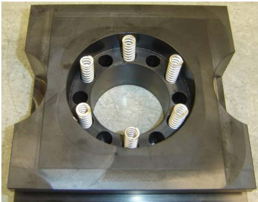
Figure 5.5. Springs in Place
