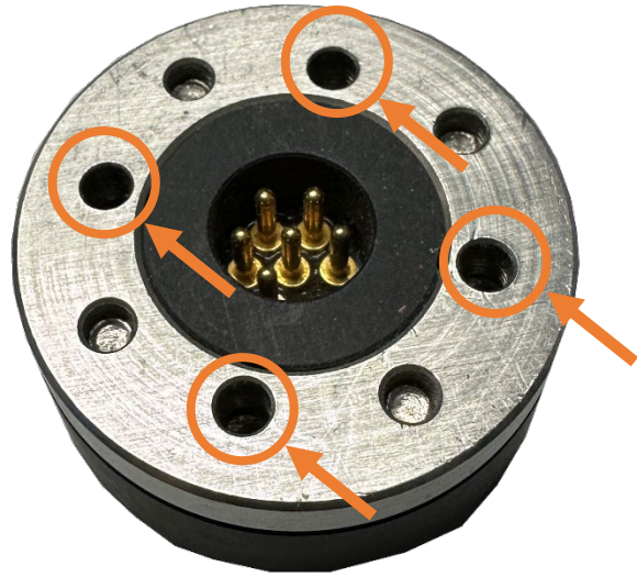
Location of the set screws attaching the Bulkhead Connector
