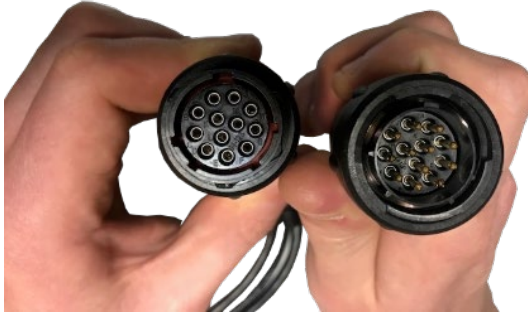
Female connector of the breakout assembly and male connector of the test cable
