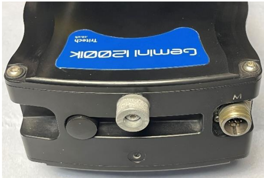
Anode in good condition.
