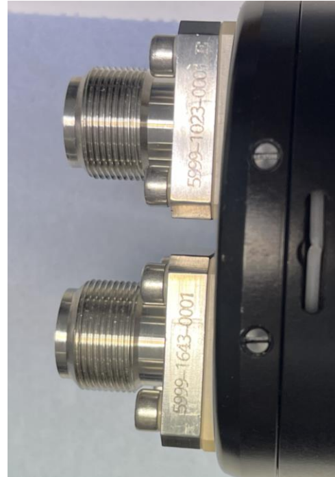
Burton 55 series connectors fitted to an older Gemini 720i's sonar
