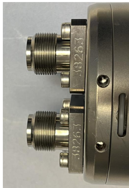
Seacon 55 series connectors fitted to a Gemini 720is sonar
