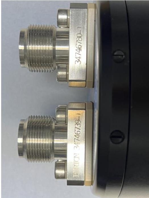
Burton 55 series connectors fitted to an older Gemini 720i's sonar
