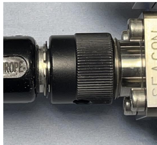
Seacon 55 series cable connector, and made up to the flange connector.
