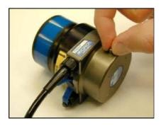
4.6.4. In Seanet Pro, select Applications > Setup. The 'MINIMODEM' type should now appear in the SeaNet Pro node table (Note: the status may be red, this indicates an update is required). If this does not happen try turning the magnet round to use the other pole and cycling the power (the magnetic sensor is uni-polar).
