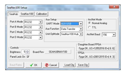
In the Aux Setup section, select UART Mode **AUX-USB**, and Aux Function **Data Transfer**. Note that this will disable the RAT (Remote Access Terminal) port on the front of the Micron Nav Hub, since the internal comms channel is reassigned to support Data Transfer.
