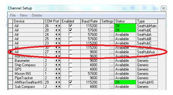
The Micron Nav Hub Aux Port is available to Windows as a generic COM port, and is the port which will be used for data transfer. In Seanet Pro -> Utilities -> Com Setup, make sure that the Enabled checkbox for this port is NOT checked; this will ensure that this port remains free for the user's application to connect to. The Baud rate to be used in the user's application is 9600 Baud.
