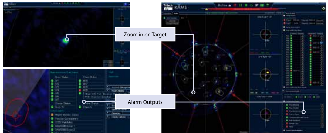
RAMS® real-time display and status overview of turret and all mooring lines, risers and umbilicals.
